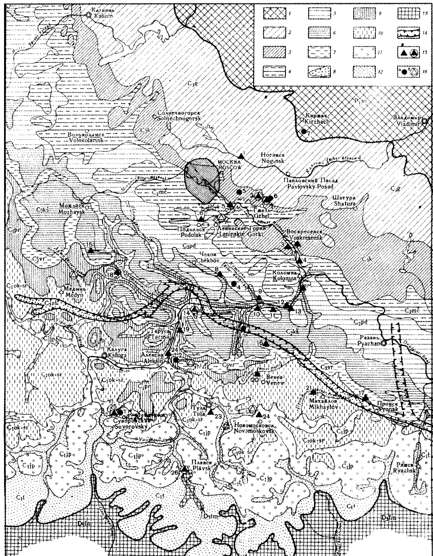
Fig. 2. Schematic geological map of the pre-Mesozoic of the south part of the Moscow Syncline and location of the most important type and reference sections (modified from Yablokov, 1975). 1 – Lower Permian, Asselian ( P_1as ); 2, 3 – Upper Carboniferous: 2 – Gzhelian ( C_3g ); 3 – Kasimovian ( C_3k ); 4–8 – Middle Carboniferous: 4–7 – Moscovian: 4 – Myachkovian ( C_2mč ); 5 – Podolskian ( C_2pd ); 6 – Kashirian ( C_2kš ); 7 – Vereian ( C_2vr ); 8 – Bashkirian, Melekessian, Aza Group ( C_2as ); 9–12 – Lower Carboniferous: 9 – Upper Serpukhovian, Protvian ( C_1pr ); 10 – Upper Visean and Lower Serpukhovian (Tarusian and Steshevian) ( C_1ok+sr ); 11 – Middle Visean, Bobrikian ( C_1jp ); 12 – Tournaisian ( C_1t ); 13 – Upper Devonian, Famennian ( D_3fm ); 14 – buried valley filled with estuarine and fluvial sediments of the Bashkirian Aza Group; 15 – type and reference sections in outcrops, numbers on the map: 1 – Stshelkovo; 2 – Gzhel; 3 – Afanasievo; 4 – Peski; 5 – Myachkovo; 6 – Podolsk; 7 – Stshurovo; 8 – Lopasnya River; 9–13 – Kashira and Gorya area; 14 – Skniga River; 15 – Vereia; 16 – Nevezhino; 17 – Alyutovo; 18 – Protva River, Rostsha; 19 – Tarusa; 20 – Venev; 21 – Mikhailov; 22 – Aleksin; 23 – Tula; 24 – Novomoskovsk (Bobriki); 25 – Cherepet River; 26 – Plavsk; 27 – Zaborie; 28 – Dashkovka; 29 – Domodedovo; 30 – Rusavkino; 16 – bore-hole reference sections
