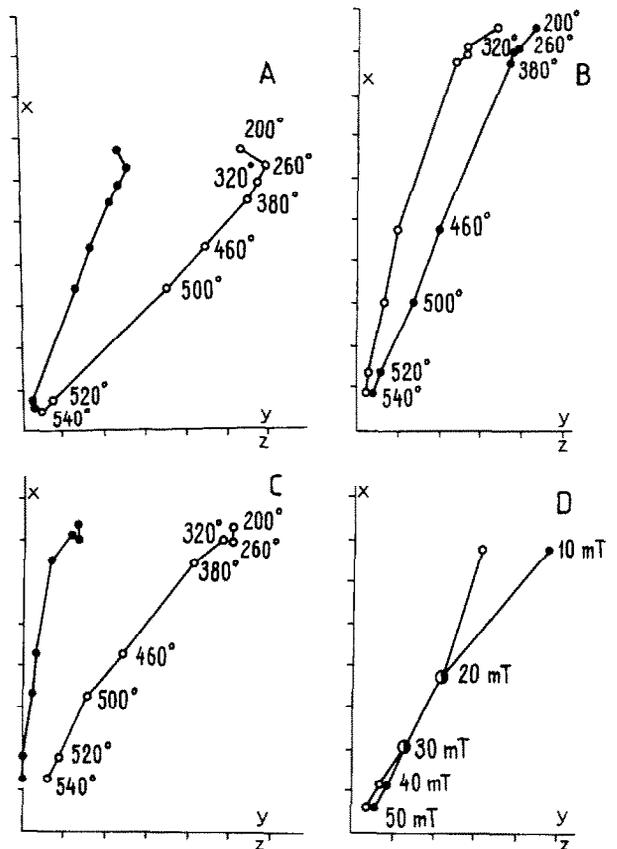
Fig. 7. Thermal (A,B,C) and a.f. (D) demagnetization of representative samples from Medny Island (locality 5); (A) sedimentary rock of the Komandorsky Formation; (B) heated host rock from the folded sill of the Medny Formation; (C, D) basalt from the same sill.
